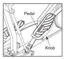
each pedal. Slide the pedals forward or backward to the desired position, and then retighten the knobs. Make sure that both pedals are in the same position.
