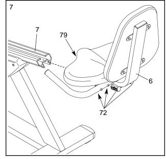
Position the Seat Carriage (6) as shown. Slide the Seat Rail Cover (84) into the slot in the Seat Rail (7). The beveled end of the Seat Rail Cover should be flush with the end of the Seat Rail. Attach a Seat Stop (77) and the Seat Rail Cover to the Seat Rail (7) with an M4 x 16mm Screw (64).
