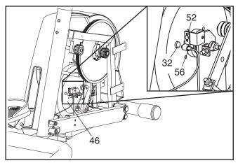
Turn the Flywheel (46) until the Magnet (32) is aligned with the Reed Switch (56) (refer to the inset drawing). Loosen the indicated Screw (52). Slide the Reed Switch slightly closer to the Flywheel, and retighten the Screw. Make sure that the Magnet will not hit the Reed Switch when the Flywheel turns. Repeat until the console displays correct feedback.
