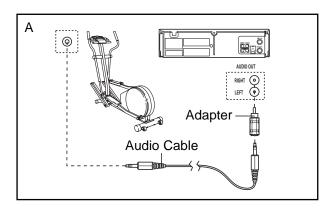
B. Plug one end of the audio cable into the jack beneath the console. Plug the other end of the cable into the adapter. Plug the adapter into an RCA Y-adapter (available at electronics stores).
