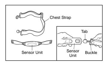
Refer to the inset drawing above. Insert the tab on one end of the chest strap through one end of the sensor unit as shown. Then, press the end of the sensor unit under the buckle on the chest strap.
