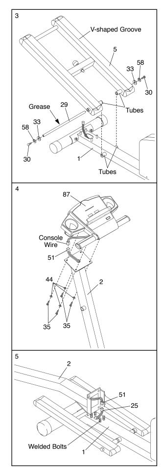
6. Align the two holes in the front of the Upright (2) with the two welded bolts on the front of the Frame (1).
