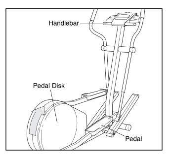
To dismount the elliptical crosstrainer, wait until the pedals come to a complete stop. **Note: The elliptical crosstrainer does not have a freewheel; the pedals will continue to move until the flywheel stops.** When the pedals are stationary, step off the highest pedal first. Then, step off the lowest pedal.
