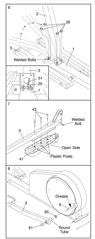
Apply grease to the welded bolt on the Left Pedal Arm
