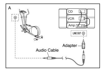
B. Plug one end of the audio cable into the jack beneath the console of the elliptical crosstrainer. Plug the other end of the cable into the included adapter. Plug the adapter into an RCA Y-adapter (available at electronics stores). Next, remove the wire that is currently plugged into the LINE OUT jack on your stereo and plug the wire into the unused side of the RCA Y-adapter. Plug the RCA Y-adapter into the LINE OUT jack on your stereo.
