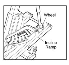
wheels make contact with it. Other parts of the elliptical crosstrainer can also be cleaned in this way. **Never use abrasives or solvents.**
