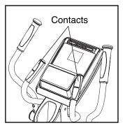
hold the handgrip pulse sensor with your palms resting against the metal contacts. **Avoid moving** your hands or gripping the contacts tightly.
