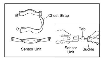
See the inset drawing above. Insert the tab on one end of the chest strap through the hole in one end of the sensor unit as shown.
