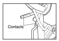
hands on the handgrip pulse sensor, with your palms on the contacts. **Avoid moving your hands.** When your pulse is detected, one or two dashes will appear in the Pulse display and then your heart rate will be shown.
