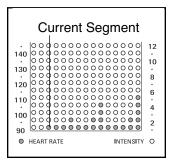
When only three seconds remain in the first segment of the program, both the Current Segment column and the column to the right will flash, a series of tones will sound, and all target heart rate settings will move one column to the left. The target heart rate setting for the second segment will then be shown in the flashing Current Segment column
