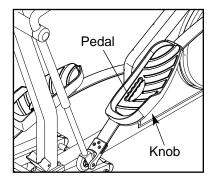
each pedal. Slide the pedals forward or backward to the desired position, and then retighten the knobs. Make sure that both pedals are in the same position.
