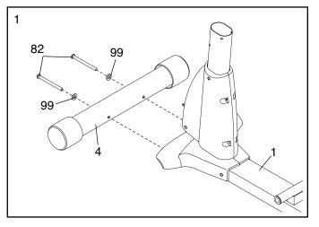
While the other person lifts the Folding Frame (2), attach the Rear Stabilizer (3) to the Folding Frame with two M10 x 93mm Button Screws (82) and two M10 Curved Washers (99). Next, tighten the Center Foot (95) into the Frame (1).
