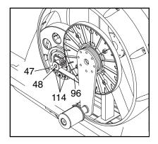
toward the rear of the elliptical exerciser until the Belt (96) is tight, and then tighten the three Button Screws.
