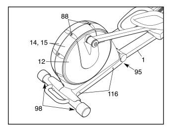
If the elliptical exerciser flexes in the center during use, turn the Center Foot (95) until the flexing is eliminated.
