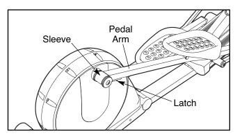
Next, raise the pedal arms until they touch the magnets on the upper body legs; the magnets will hold the pedal arms in place. Then, hold the handle and lift the frame until it locks in a vertical position.
