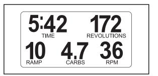
The upper right corner of the display will show the distance you have pedaled, in total revolutions. The display will also show your heart rate when you use the handgrip pulse sensor (see step 5 on page 14).
