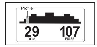
During both programs, the console will regularly compare your heart rate to the target heart rate setting for the current segment of the program. If your heart rate is too far below or above the target heart rate setting, the resistance of the pedals will automatically increase or decrease to bring your heart rate closer to the target heart rate setting. Each time the resistance changes, the resistance level will appear in the display for a few seconds to alert you.
