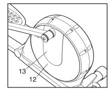
Cover (13) using a flat screwdriver. Next, remove the four screws (not shown) from the center of the left Disc (12). Gently rotate the Disc Cover and the Disc away from the elliptical exerciser.
