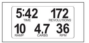
The upper right corner of the display will show the distance you have pedaled, in total revolutions. The display will also show your heart rate when you use the handgrip pulse sensor (see step 5 on page 15).
