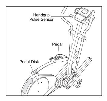
To dismount the elliptical crosstrainer, wait until the pedals come to a complete stop. The elliptical crosstrainer does not have a free wheel; the pedals will continue to move until the flywheel stops. When the pedals are stationary, step off the highest pedal first. Then, step off the lowest pedal.
