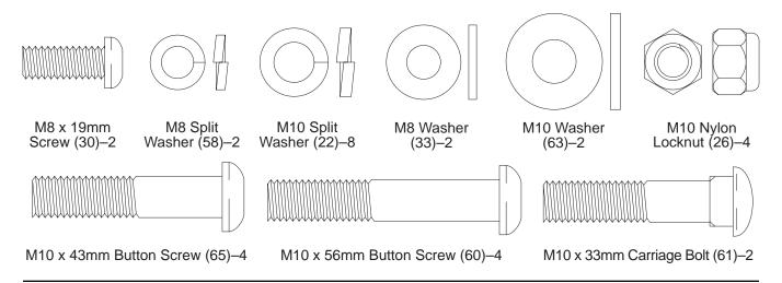
Identify the Rear Stabilizer (59), which has Leveling Feet (14) threaded into it. Attach the Rear Stabilizer to the Frame with the four M10 x 56mm Button Screws (60) and four M10 Split Washers (22).
