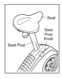
slide the seat post upward or downward to the desired position, and then release the knob. Move the seat post up or down slightly to make sure that the knob is engaged in one of the adjustment holes in the seat post. Then, turn the knob clockwise to tighten it.
