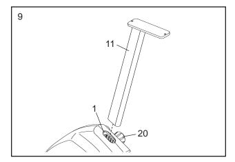
10. Attach an M6 x 10mm Screw (60) to the Seat Post (11). Next, slide the Seat Carriage (19) onto the Seat Post. Then, adjust the Seat Carriage to the desired position and tighten the Seat Knob (31) into the Seat Carriage.
