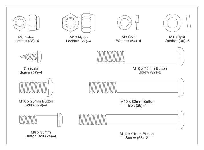
While another person lifts and holds the indicated end of the Frame (1), attach the Front Stabilizer (95) to the Frame with two M10 x 75mm Button Screws (92).
