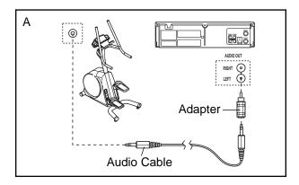
B. Plug one end of the audio cable into the jack beneath the console of the stepper. Plug the other end of the cable into the included adapter. Plug the adapter into an RCA adapter (available at electronics stores). Next, remove the wire that is currently plugged into the AUDIO OUT jack on your VCR and plug the wire into the unused side of the RCA adapter. Plug the RCA adapter into the AUDIO OUT jack on your VCR.
