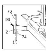
bent end of the Leg Pin points toward the floor. Rotate the Leg Pin to secure it around the Leg. Retighten the Incline Knob.
