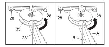
Cord over the hip pad. Make sure that the ends of the Arm Cord are even.
