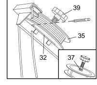
roughen the surface of the leather Resistance Pad (32) with 100-grit sandpaper or a file.
