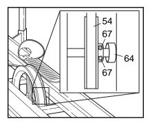
ly with a wrench. CAUTION: Do not overtighten the Nuts; this can break the "U" Bolt.
