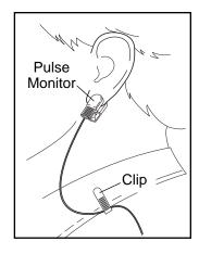
clothes clip onto your collar to prevent excessive movement of the wire.
