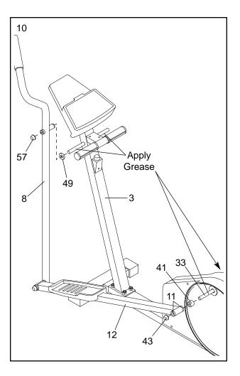
11. Make sure that all parts of the elliptical exerciser are properly tightened. Note: Some hardware may be left over after assembly is completed. To protect the floor or carpet from damage, place a mat under the elliptical exerciser.
