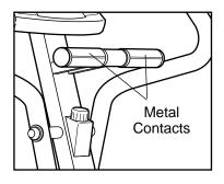
touching the lower contacts. Avoid moving your hands. After a moment, the heart-shaped indicator in the display will begin to flash and your heart rate will be shown. For the most accurate heart rate reading, continue to hold the contacts for about 15 seconds.
