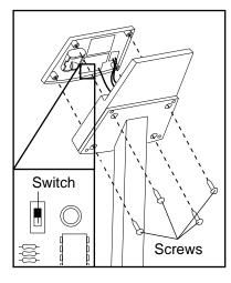
console. Slide the switch up or down to change the unit of measurement. Reattach the console with the four screws; be careful not to pinch any of the wires.
