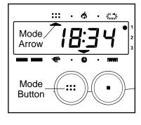
display the speed, time, distance, lap and calorie modes, for 5 seconds each, in a repeating cycle.
