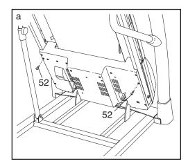
Remove the four #8 x 3/4" Screws (14) and carefully remove the Motor Hood (61).
