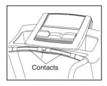
To measure your heart rate, stand on the foot rails and hold the contacts—avoid moving your hands. When your pulse is detected, your heart rate will be shown. For the most accurate heart rate reading, continue to hold the contacts for about 15 seconds.
