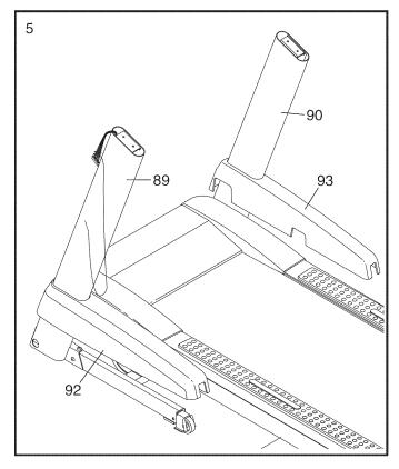
6. With the help of a second person, hold the console assembly near the Left Upright (89).
