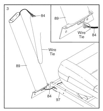
Hold the Left Upright (89) against the Base (97). Be careful not to pinch the wires. If necessary, position the Base Ground Wire (94) in the hole in the side of the Left Upright. Insert two 3/8" x 2 3/4" Bolts (7) and two 3/8" x 1 1/4" Bolts (8) with two 3/8" Star Washers (12) into the Left Upright.
