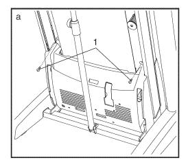
Lower the treadmill (see HOW TO LOWER THE TREADMILL FOR USE on page 28). Remove the three #8 x 3/4" Screws (1). Carefully pivot the Motor Hood (71) off.
