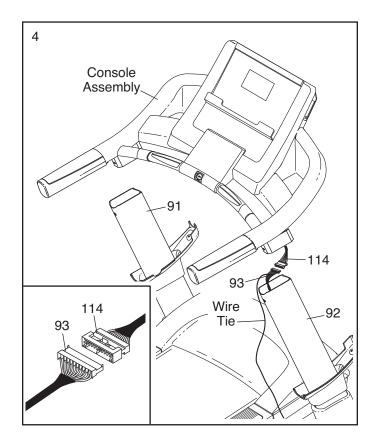
Insert the brackets on the Handrail (110) into the Uprights (91, 92). Make sure that no wires are pinched.
