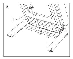
Lower the treadmill (see HOW TO LOWER THE TREADMILL FOR USE on page 24). Remove the four indicated #8 x 3/4" Screws (1), and remove the Motor Hood (75).
