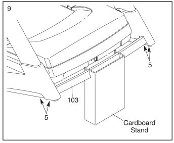
10. Make sure that all parts are properly tightened before you use the treadmill. Keep the included hex keys in a secure place; one of the hex keys is used to adjust the walking belt (see pages 26 and 27). To protect the floor or carpet from damage, place a mat under the treadmill. Extra hardware may be included.
