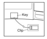
light. IMPORTANT: In an emergency, the key can be pulled from the console, causing the walking belt to slow to a stop. Test the clip by carefully taking a few steps backward; if the key is not pulled from the console, adjust the position of the clip.
