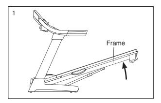
2. Raise the frame until the latch knob locks in the storage position. **CAUTION:** Make sure that the latch knob locks.
