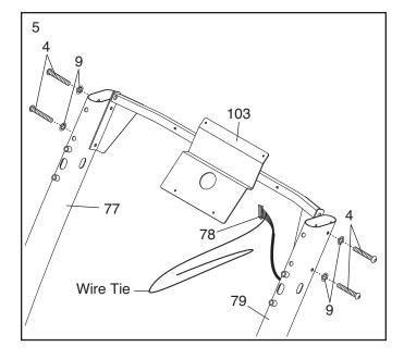
Set the Console Cover (87) on the Uprights (77, 79). Make sure that the Console Cover is oriented with the ties toward the bottom as shown.
