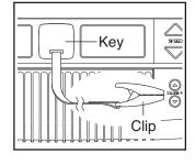
the displays will light. **IMPORTANT: In an emergency**, the key can be pulled from the console, causing the walking belt to slow to a stop. Test the clip by carefully taking a few steps backward; if the key is not pulled from the console, adjust the position of the clip.
