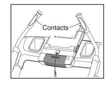
To measure your heart rate, **stand on the walking platform** and hold the metal contacts on the handrail for approximately ten seconds—**avoid moving your hands.** When your pulse is detected, your heart rate will be shown. For the most accurate heart rate reading, continue to hold the contacts for about 15 seconds.
