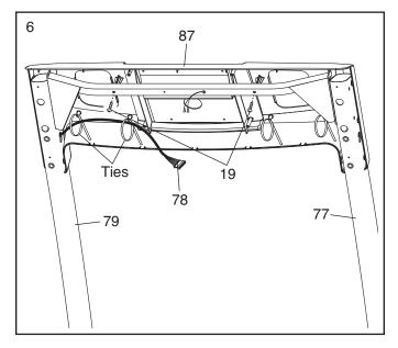
7. Have a second person hold the Left Pulse Handrail (86) near the Left Upright (77). Insert the Left Pulse Wire (90) from the Left Pulse Handrail through the hole in the Left Upright and out of the hole in the side of the Left Upright. Then, insert the Left Pulse Wire through the loops in the ties.
