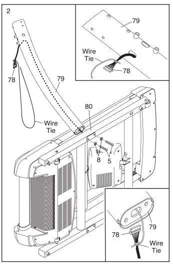
3. With the help of a second person, carefully tip the incline trainer down so that the Base (80) is flat on the floor.
