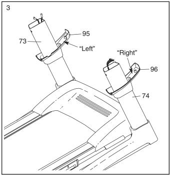
4. With the help of a second person, hold the console assembly near the Uprights (73, 74).
