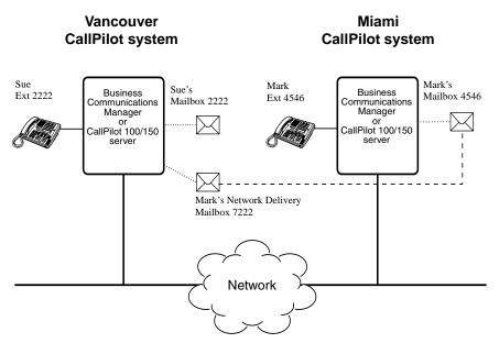
The diagram Sending a network message shows how messages are sent between different company sites on the same network. In the example, Sue works in the Vancouver office and Mark works in the Miami office.
