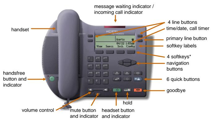
\*The four soft keys under the LCD display also allow you to access many additional features (as detailed in the IP Phone 2002 User Guide).
