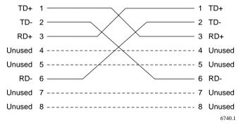
Figure 4. 10BASE-T Ethernet UTP crossover cable pin assignments
