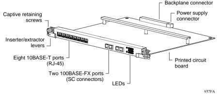
Figure 1. EtherSpeed 10BASE-T/100BASE-FX Switch Module
