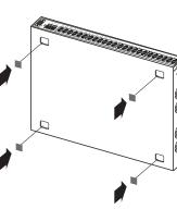
5. Set the device on a flat surface near an AC power source, making sure there are at least 2 inches (5.1 cm) of space on all sides for proper air flow and at least 5 inches (12.7 cm) at the back for power cord clearance.
