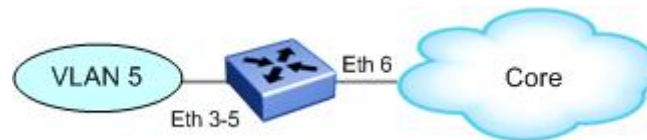
Figure 6: DSCP Mapping via Un-restricted Port Role
