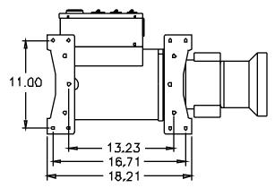
After the the generator is firmly mounted, attach the PTO driveline to the generator then the tractor. Use a synchronized PTO driveline rated at 24 HP minimum.
