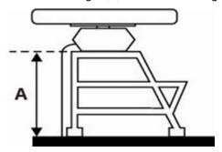
If the trestle height (A) is more than 2 m high, install a radar mast secured with guy wires as shown:
