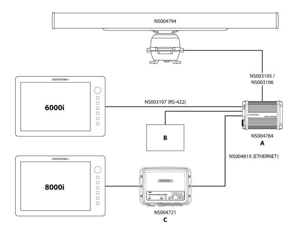
where A is the radar processor, B is the vessel's power supply (24 V DC ONLY), and C is the Network Linker (NS004721).
