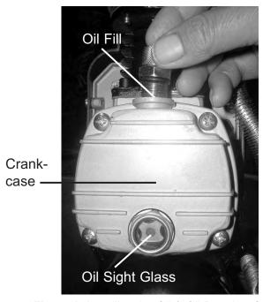
Figure 2. Installing the Oil & Oil Breather Cap
