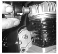
Figure 4. Installing the Air Filter
