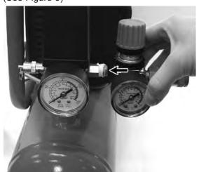
Figure 3. Installing the Air Regulator
