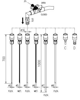
Fig.2: Connect compressed air 100PSI (7bar) to quick couple D. Open the ball
