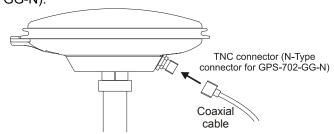
5. Attach the other end of the coaxial cable to the antenna input port of the receiving device, which must provide power as detailed in the SPECIFICATIONS section of this guide. All NovAtel GPS receivers provide the necessary power through their antenna RF connectors.
