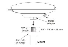
$\bowtie$ The metal adapter on the bottom of the antenna is fixed in place. Do not attempt to remove it.
