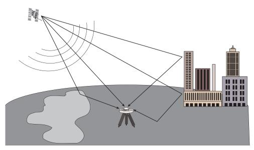
Figure 25: Illustration of GPS Signal Multipath
