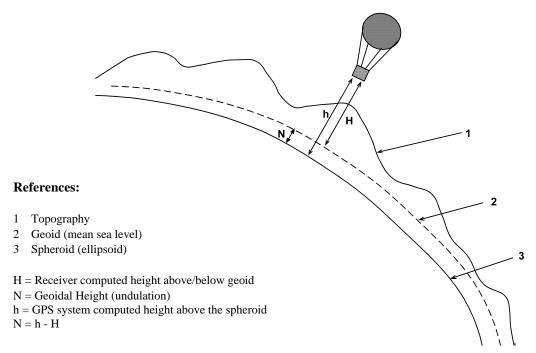
Figure 22: Illustration of Receiver Height Measurements
