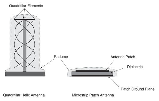
Figure 27: Illustration of Quadrifilar vs. Microstrip Patch Antennas
