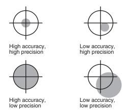
Figure 23: Accuracy versus Precision<sup>1</sup>
