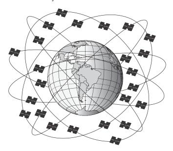
Figure 21: NAVSTAR Satellite Orbit Arrangement
