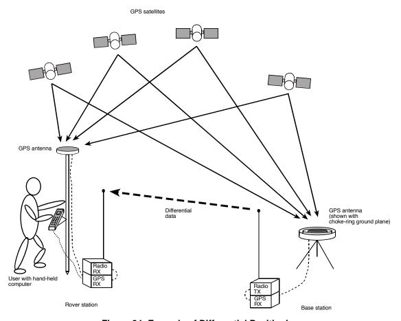
Figure 24: Example of Differential Positioning
