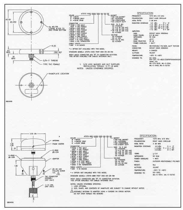
Figure 15: GPS Antenna 201-990147-432 (1575 MHz) and 201-990144-807 (Pre-Amplifier)
