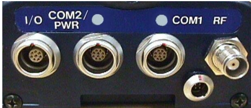
Figure 4: Close-up of Ports on Rear End-cap
