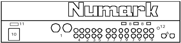
1. The **Balanced Main Outputs** are low-impedance XLR type connectors controlled by the **Master** fader.
