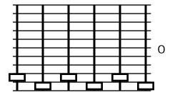
Below is the <u>worst</u> sort of curve to use because you are using EQ to *add volume*. With exaggerated boost you can easily run your power amplifiers into "clipping" (see page 6) and damage your speakers.
