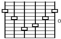
Below is an example of a poor EQ curve because it cuts the output volume down by 6-10dB. You have to compensate by running the **Master** output higher:
