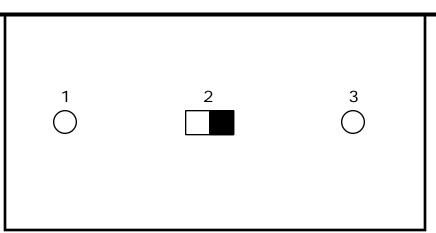
1. Microphone Jack for a 1/4" Microphone connector.
