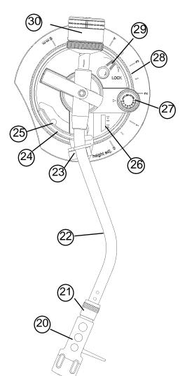
20. Headshell - Attach the cartridge here.
