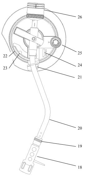
18. Headshell- Install cartridge here. When installing a cartridge, refer to the installation instructions supplied by the manufacturer of that cartridge. During installation, attach the stylus protector to guard the stylus tip from damage.
