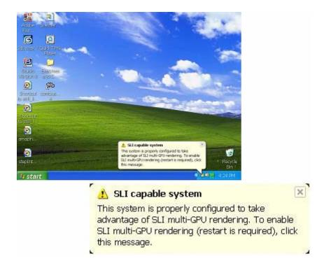
6. Click anywhere on the message above (if the message disappears, right click on the desktop and select Properties/Settings/Advanced/Quadro FX xxxx/SLI multi-GPU). Check the "Enable SLI multi-GPU" as shown in the screen capture below and select OK.
