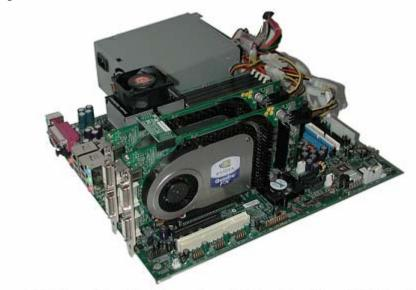
SLI Capable Configuration Using Quadro SLI Cards
