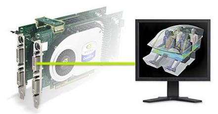
SLI Multi View: Combines the power of two NVIDIA Quadro PCI Express graphics boards to span a single hardware-accelerated OpenGL application window across multiple displays, run a single application per GPU with multiple display outputs, or enable other flexible usage of two PCI Express graphics boards.
