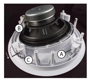
10. Your speaker includes a pivoting tweeter and it may be aimed to achieve even better imaging. Tweeter output should be directed toward the typical listening position. USE CARE TO AVOID DAMAGING THE DOME OF THE TWEETER DURING AIMING!!
