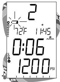
Fig. 9- Low Battery Condition
