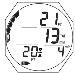
Fig. 75 - DECO STOP MAIN
