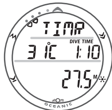
Fig. 138 - FREE DIVE MAIN (During CDT ALARM)
