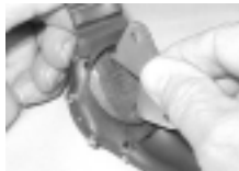
Fig. 144 - BATTERY HATCH REMOVAL (Tool)
