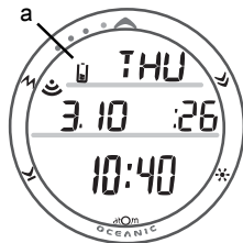
Fig. 3 - LOW BATTERY WARNING
