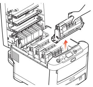
**4.** Put the assembly down gently onto a piece of paper to prevent toner from marking your furniture and to avoid damaging the green drum surface.
