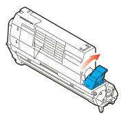
**10.** Holding the complete assembly by its top centre, lower it into place in the printer, locating the pegs at each end into their slots in the sides of the printer cavity.
