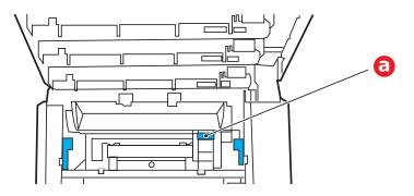
**11.** If you are not using the rear exit tray, close it once any paper has been removed from this area.
