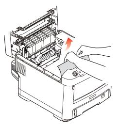
(b) To remove a sheet from the central area of the belt (2), carefully separate the sheet from the belt surface and withdraw the sheet.
