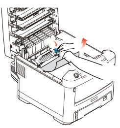
(c) To remove a sheet just entering the fuser (3), separate the trailing edge of the sheet from the belt, push the fuser pressure release lever (4) towards the front and down to release the fuser's grip on the sheet, and withdraw the
