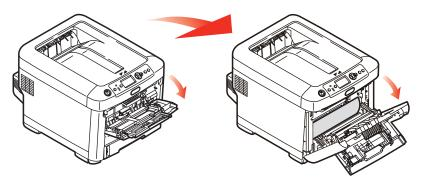
**14.** Check inside the cover for sheets in this area and remove any that you find, then close the cover.
