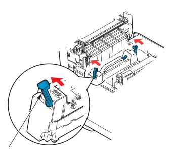
**8.** Starting with the cyan image drum unit nearest the fuser, replace the four image drums into the drum cavity, making sure to locate them in the correct order.
