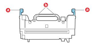
**7.** Lower the fuser into the printer, locating the two lugs (b) into their slots in the metal partition which separates the fuser area from the image drums.
