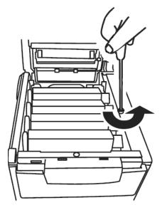
6. Lift up on the ends of the side panel, then remove it from the printer.
