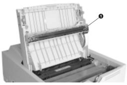
Wipe the LED array (1) gently with the cleaning pad that came with your toner cartridge. You can also use a clean, soft cloth with a small amount of rubbing alcohol on it.
