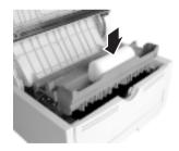
5. Remove the shipping insert from the toner well and discard. Reset the drum counter (see below), and install a new toner cartridge following the instructions in the previous section.
