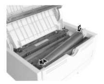
Push the coloured tab forward to release the toner into the 6. toner hopper.
