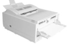
Use the front tray to feed this type of paper and the rear paper exit to collect your printed output. This gives a nearly straight paper path through the machine, and may prove more reliable in this type of application.
