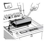
6. Reinstall the image drum cartridge back into the printer, locating the pins on each end into the slots at either side of the printer.
